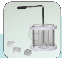
Three tube bolus basket assembly with guided disc (Set of 2) for EDI-2 / EDI-2L Part no - 0202A00010
