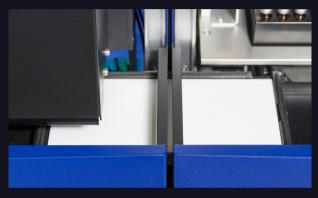
The built-in conveyor transports clean plates from the Module PLATE STORAGE to the Module APPLICATION.
