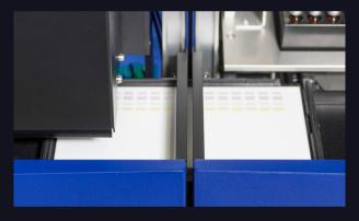
After or during analysis, the plates are transported back to the Module PLATE STORAGE.
